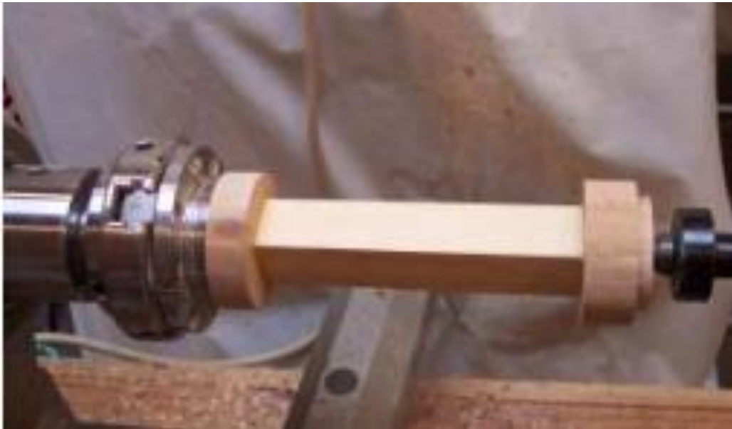
The blank with two disks glued to the ends for greater stability when threading.
