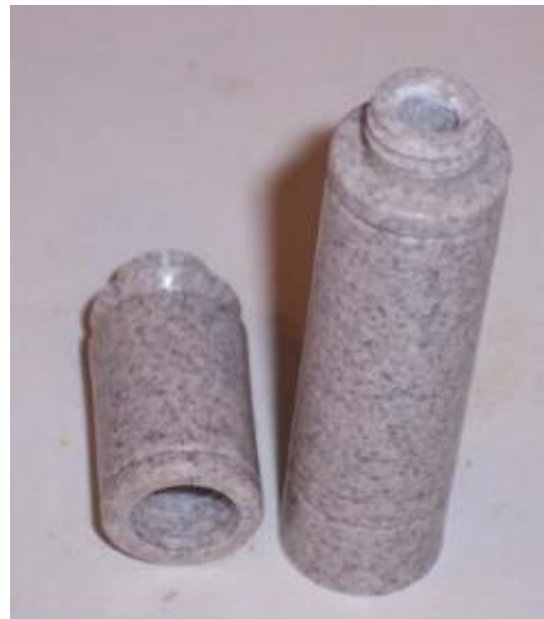
A needle case made from Corian. Corian threads very well. This one was not held with the disks, but only in the 25mm jaws of the chuck. I broke off the threaded tenon once and had to shorten the case.
