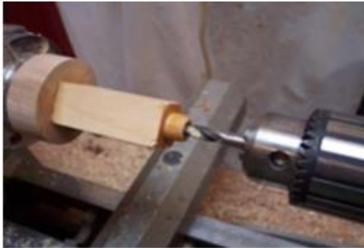
Drilling the 5/16" hole to hold the needles. It can be drilled before or after threading.
