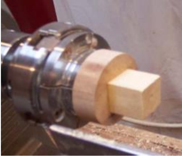
The lid is ready to drill with a 7/16" drill to a depth of about 1/2".
