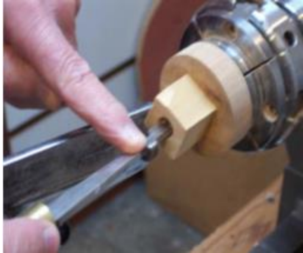
Threading the hole in the lid with the inside chasers.
